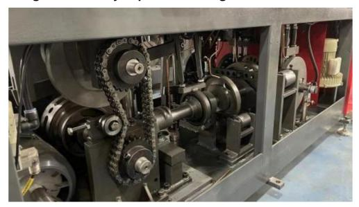
1. The whole **cup cake forming machine** adopts automatic oil lubrication system( oil circulation system is including oil motor, filter, copper pipe) which makes all gear moving parts working at high speed much more smoothly and greatly Improve the service life of spare parts.
